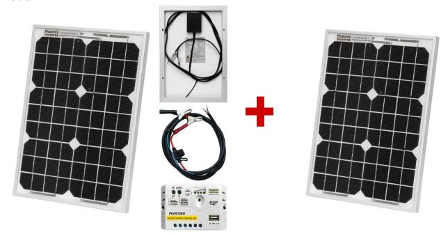
Connect the second 10W solar panel to the same solar terminals of the charge controller, in parallel with your existing 10W solar panel (connecting "+" to "+", "-" to "-") – it's that simple. **The output of your solar kit will double and the charging time will halve.**
