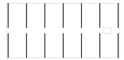
If your solar panel width (and the length of each adhesive line) is greater than 600 mm, break the adhesive lines in the middle of the solar panel with a gap of 30-40 mm to allow for additional escape routes for air and rain water.
