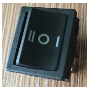
“I” – inverter is On
