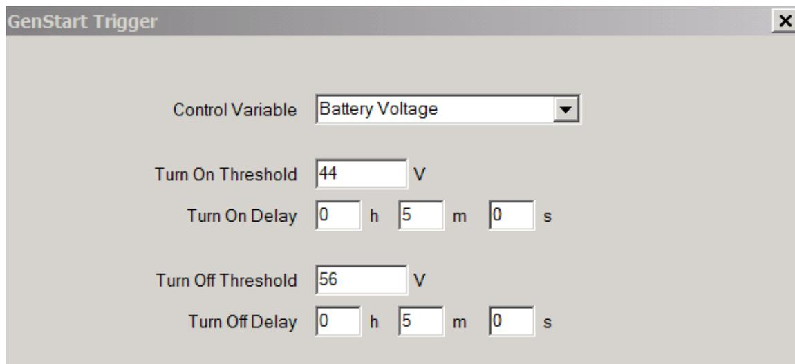
Fig. 6 Battery Thresholds
