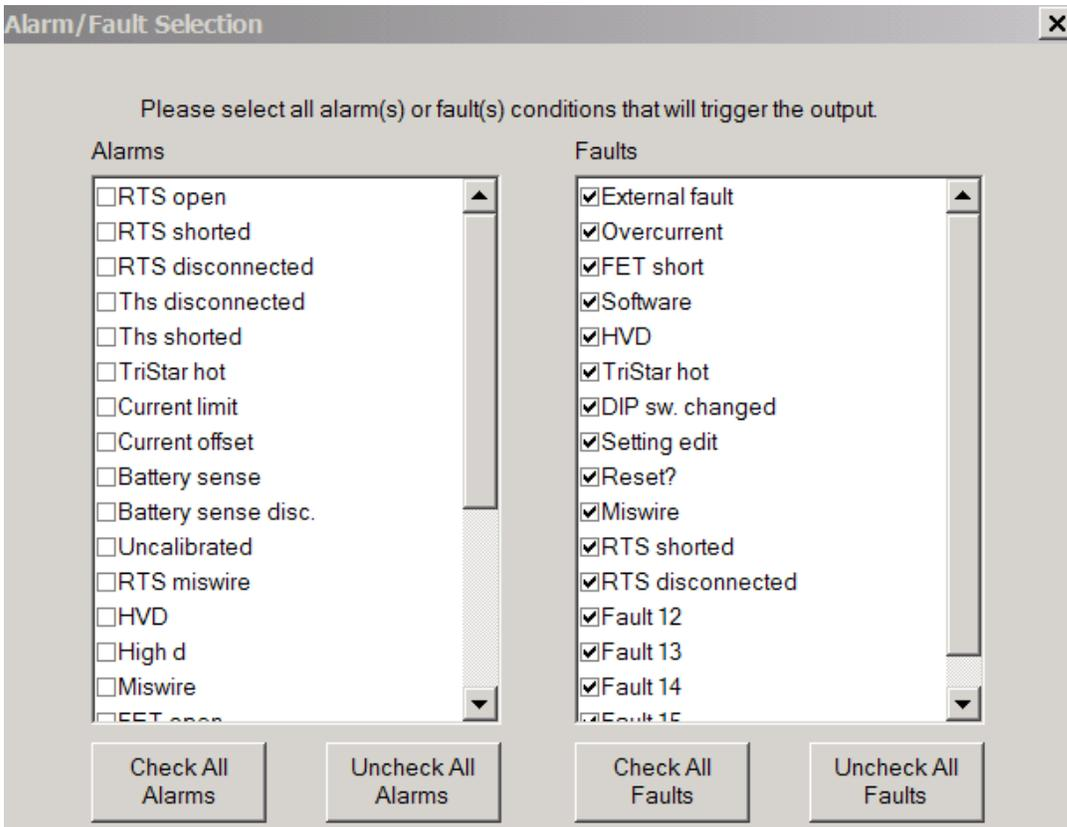
Fig. 3 TriStar Alarm and Fault Selection
