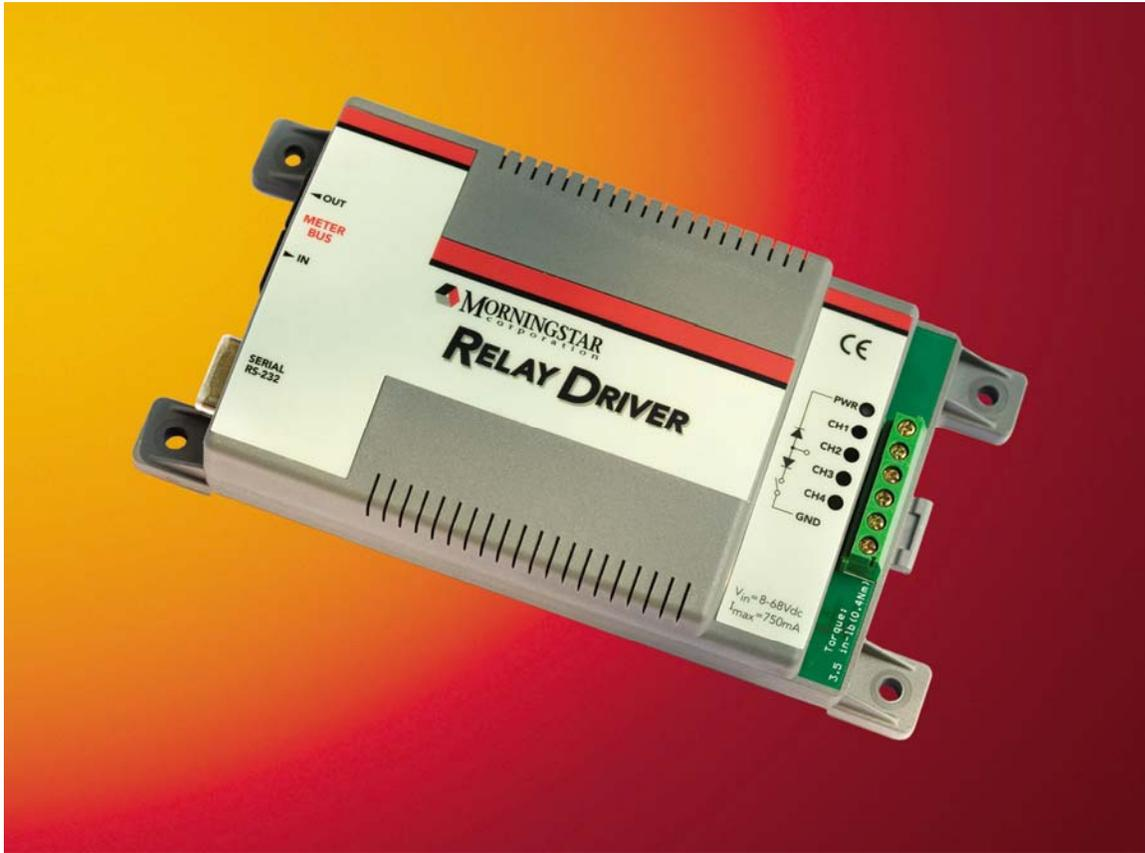
Morningstar's Relay Driver (RD) is a fully programmable 4-channel logic controller that can be used to control mechanical or solid-state relays in an AC or DC power system. A limitless number of combinations can be configured for each channel on the RD to control the switching of circuits on and off based on several variables present in the system. The purpose of this document is to explore three of the many applications and uses of this product:
