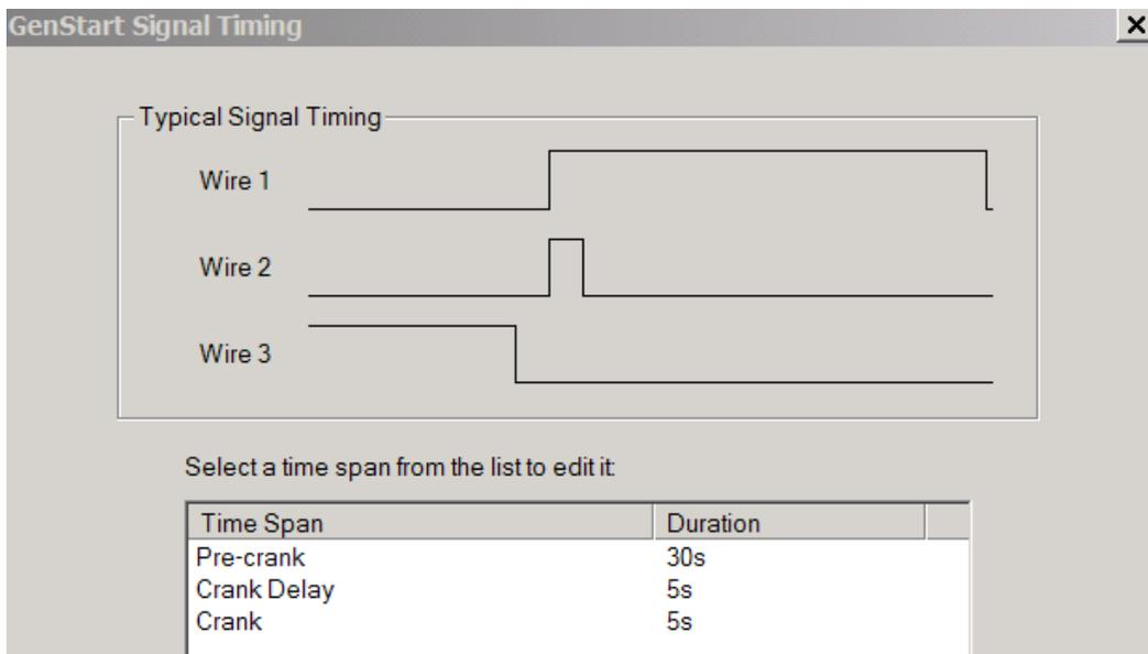
Fig. 7 Generator Starting Cycle
