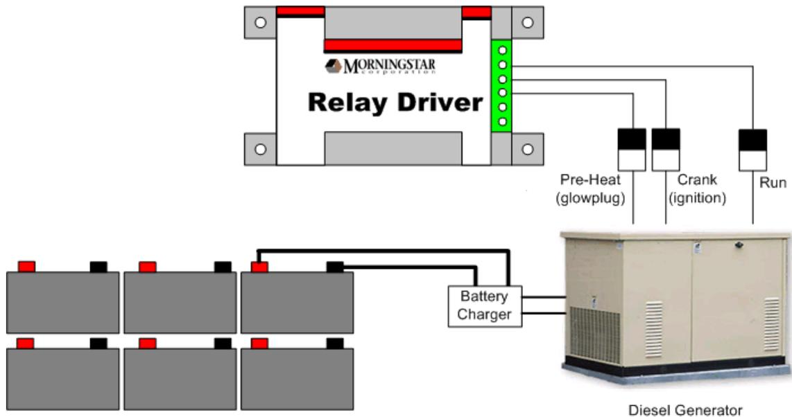
The first set up is the generator start and stop. In stand alone mode, the Relay Driver accomplishes this with battery voltage readings (taken at its own power terminals) as shown in Fig 6.
