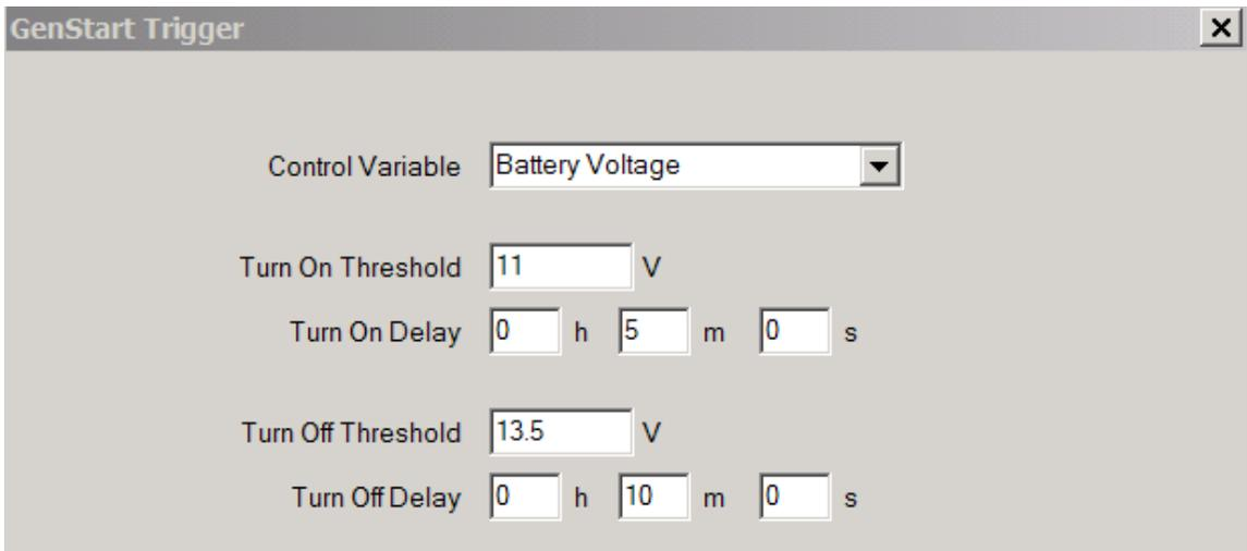
Fig. 2 Voltage Threshold Setup for Genstart
