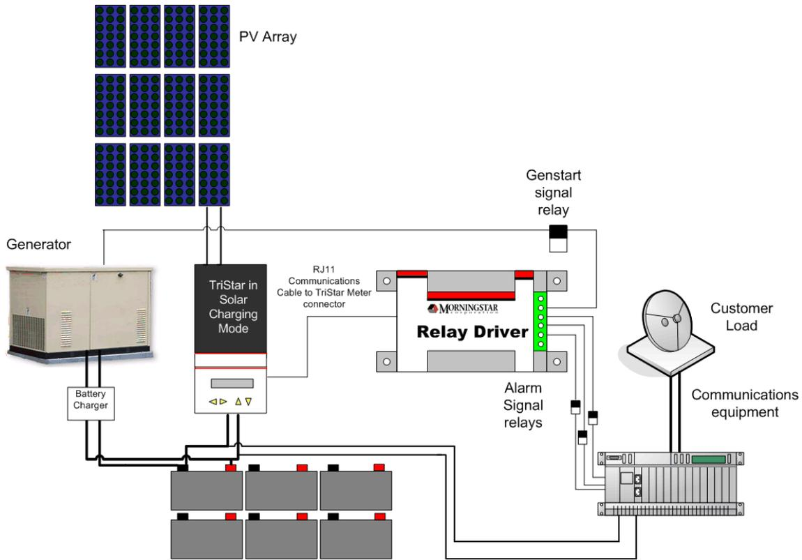
In this application, the Relay Driver is used to send voltage alarms to a communications device provided by the user at the site. It also will monitor battery voltage and start a generator whenever there is insufficient solar charging from the PV array.
