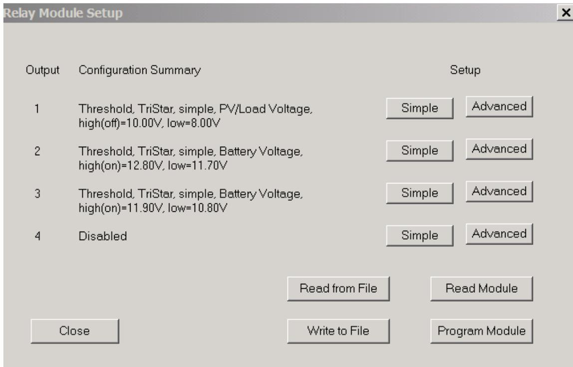
Fig. 5 Lighting Control Thresholds
