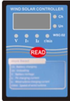
Pressing “**READ**” on the controller will show the battery voltage, solar charge current, wind turbine charge current and wind turbine revolutions per minute (RPM).
