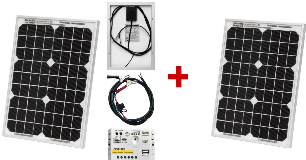
Connect the second 10W solar panel to the same solar terminals of the charge controller, in parallel with your existing 10W solar panel (connecting “+” to “+”, “-” to “-”) – it’s that simple. **The output of your solar kit will double and the charging time will halve.**
