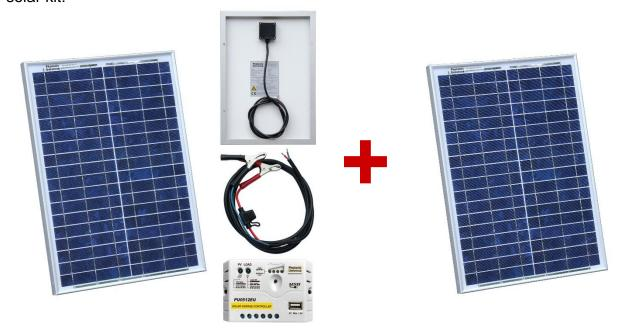
Connect the second 20W solar panel to the same solar terminals of the controller, in parallel with your existing 20W solar panel (connecting "+" to "+", "-" to "-") – it's that simple. The output of your solar kit will double and the charging time will halve.
