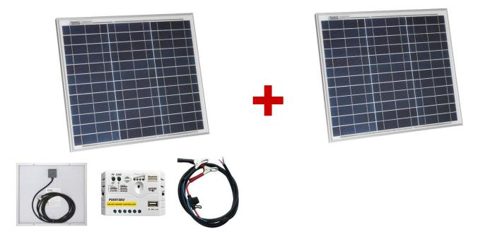
Connect the second 30W solar panel to the same solar terminals of the controller, in parallel with your existing 30W solar panel (connecting "+" to "+", "-" to "-") – it's that simple. The output of your solar kit will double and the charging time will halve.
