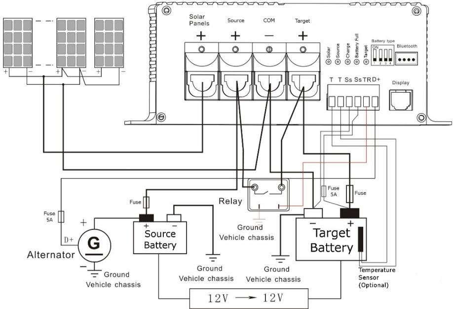
Connection diagram for DC1224-2530, DC2424-5030 & DC2412-6050:
