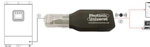
① Connect the WiFi adapter to the RJ45 port of the device. ② Add the WiFi adapter into the cloud by the PC or mobile app. **WARNING: The WiFi adapter is not compatible with the PU1024B/PU2024B, PU1024BW/PU2024BW and LS-B series controllers. If the WiFi adapter is installed in a metal cabinet, the signal strength and distance will be reduced, depending on the material and size of the cabinet.**
