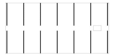
If your solar panel width (and the length of each adhesive line) is greater than 600 mm, break the adhesive lines in the middle of the solar panel with a gap of at least 100 mm to allow for additional escape routes for air and rain water.
