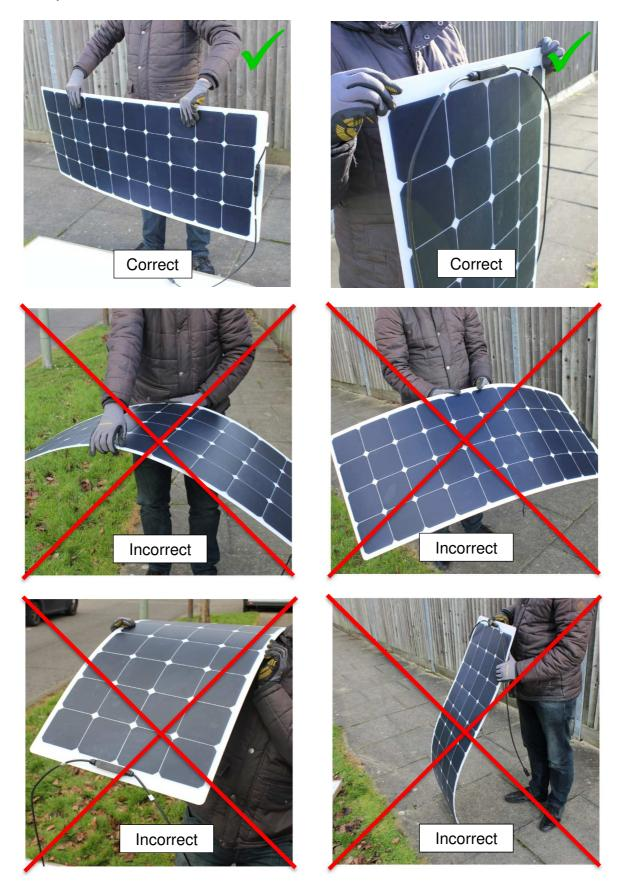
Never attempt to test the "local flexibility" of the solar panel by bending the material of the solar panel near the edges or in the corners. This can easily cause solar cell cracks.
