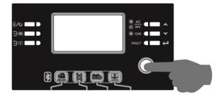
Step 4. Be sure to select battery type as "SOL" in LCD program 5.
