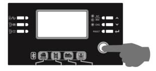
Step 4. Be sure to select battery type as "WEC" in LCD program 5.
