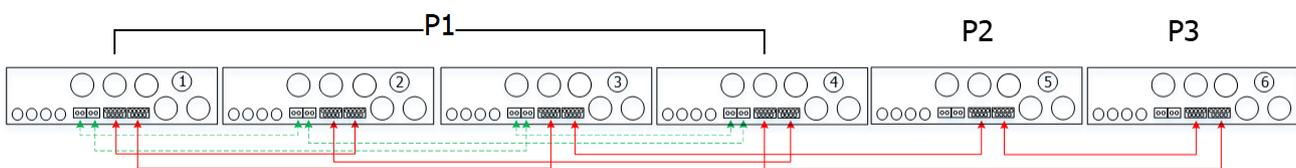
Three inverters in one phase, two inverters in second phase and one inverter for the third phase:
