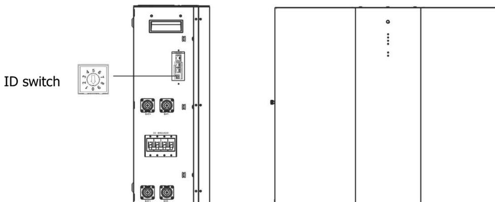
ID Switch indicates the unique ID code for each battery module. It's required to assign a unique ID to each battery module for normal operation. We can set up the ID code for each battery module by rotating the PIN number on the ID switch. From number 0 to 9, the number can be random; no particular order. Maximum 10 battery modules can be operated in parallel.
