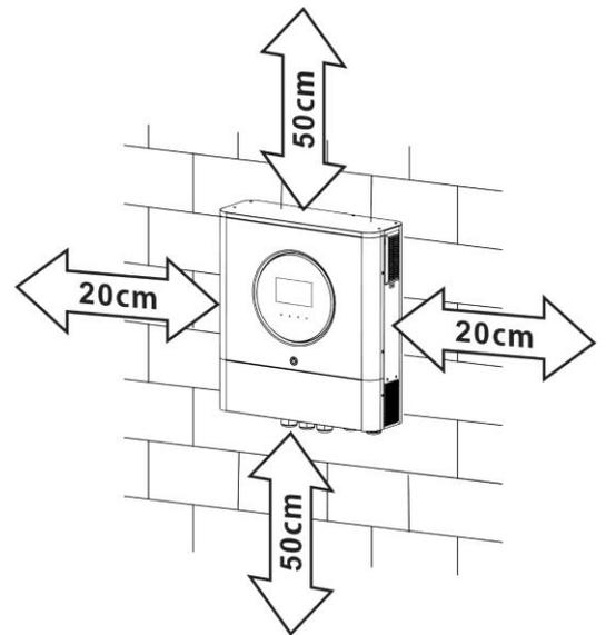
**⚠ SUITABLE FOR MOUNTING ON CONCRETE OR OTHER NON-COMBUSTIBLE SURFACE ONLY.**
