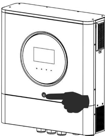
Step 5. Be sure to select battery type as "PYL" in LCD program 5.
