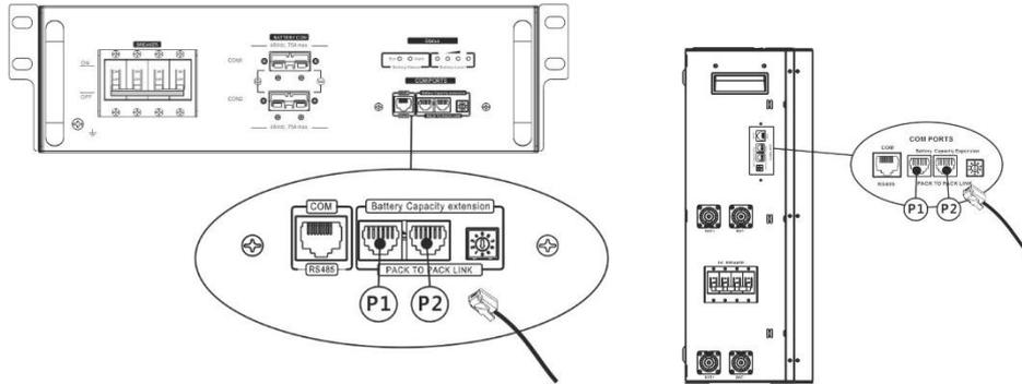
Step 2: Use supplied RJ45 cable (from battery module package) to connect inverter and Lithium battery.
