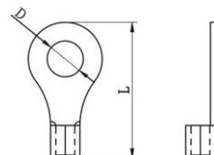
**Recommended battery cable and terminal size:**
