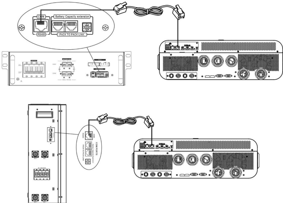
\* For multiple battery connection, please check battery manual for the details.
