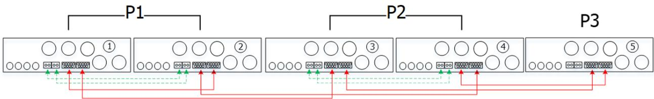
Two inverters in one phase and only one inverter for the remaining phases:
