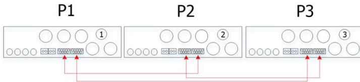
**WARNING:** Do not connect the current sharing cable between the inverters which are in different phases. Otherwise, it may damage the inverters.
