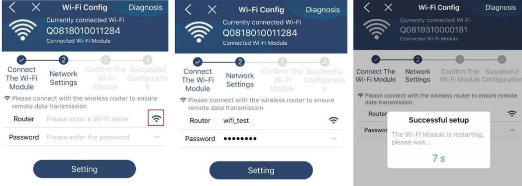
Step 4: Tap "Confirm" to complete the Wi-Fi configuration between the Wi-Fi module and the Internet.
