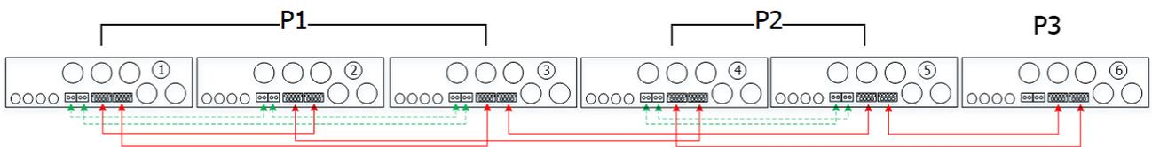
Three inverters in one phase and only one inverter for the remaining two phases:
