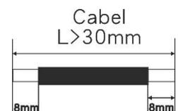
Insert striped cable into female terminal and crimp female terminal as shown below.
