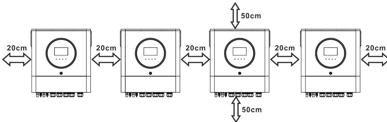
**NOTE:** For proper air circulation to dissipate heat, allow a clearance of approx. 20 cm to the side and approx. 50 cm above and below the unit. Be sure to install each unit in the same level.
