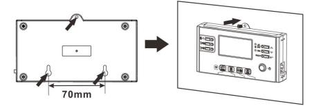
**Note:** Installation to the wall should be implemented with the proper screws. Refer chart for recommended spec of screws.
