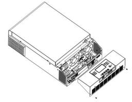
**Step 2:** Remove two screws as below chart and remove 2-pin and 14-pin cables.
