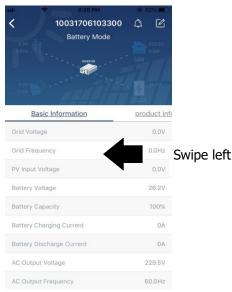
**[Basic Information]** displays basic information of the inverter, including AC voltage, AC frequency, PV input voltage, Battery voltage, Battery capacity, Charging current, Output voltage, Output frequency, Output apparent power, Output active power and Load percent. Please slide up to see more basic information.
