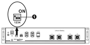
• ADD Switch: There are 4 ADD switches are to define different baud rate and battery group address. If switch position is turned to bottom for "OFF" position, it means "0". If switch position is turned to upper for "ON" position, it means "1".
