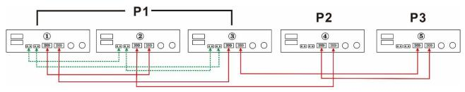
Two inverters in two phases and only one inverter for the remaining phase:
