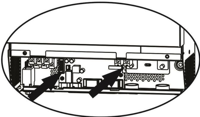
**Step 5:** Re-connect 2-pin and 14-pin to original position on parallel board as shown below chart.
