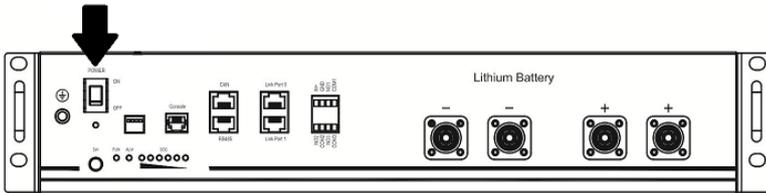
Step 3. Press more than three seconds to start Lithium battery. Output power is ready.
