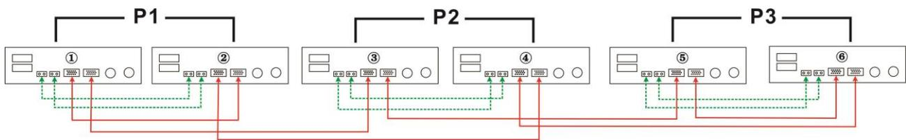
Four inverters in one phase and one inverter for the other two phases:
