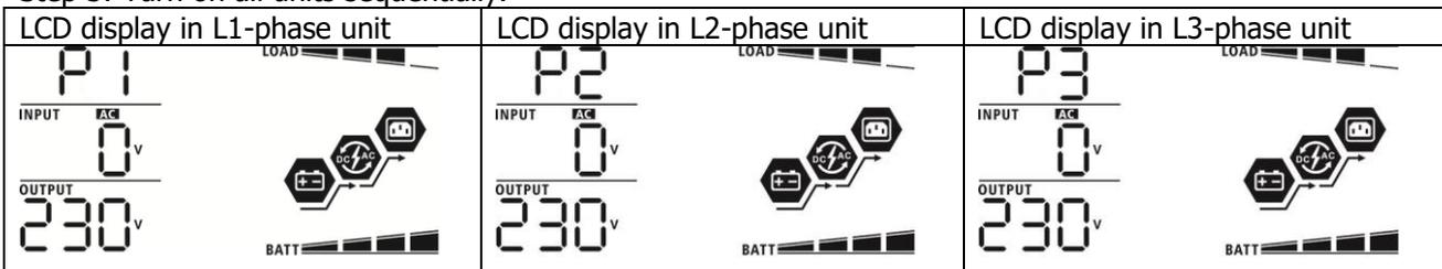
Step 4: Switch on all AC breakers of Line wires in AC input. If AC connection is detected and three phases are matched with unit setting, they will work normally. Otherwise, the AC icon will flash and they will not work in line mode.
