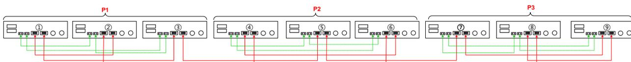
**Note:** If there is only one unit in one phase, this unit doesn't need to connect the current sharing cable.
