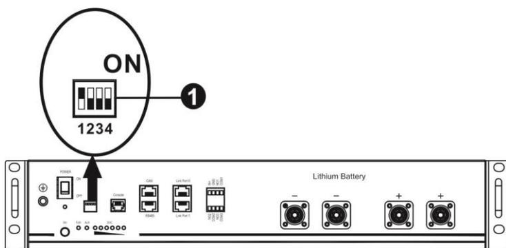
① ADD Switch: There are 4 ADD switches are to define different baud rate and battery group address. If switch position is turned to bottom for "OFF" position, it means "0". If switch position is turned to upper for "ON" position, it means "1".
