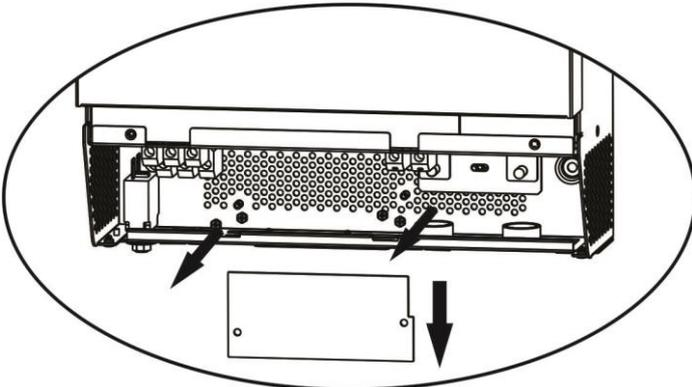
**Step 3:** Remove two screws as below chart to take out cover of parallel communication.
