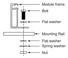
• Four M8(5/16inch) stainless steel bolts, four nuts, four spring washers, and eight flat washers are recommended per solar module.
