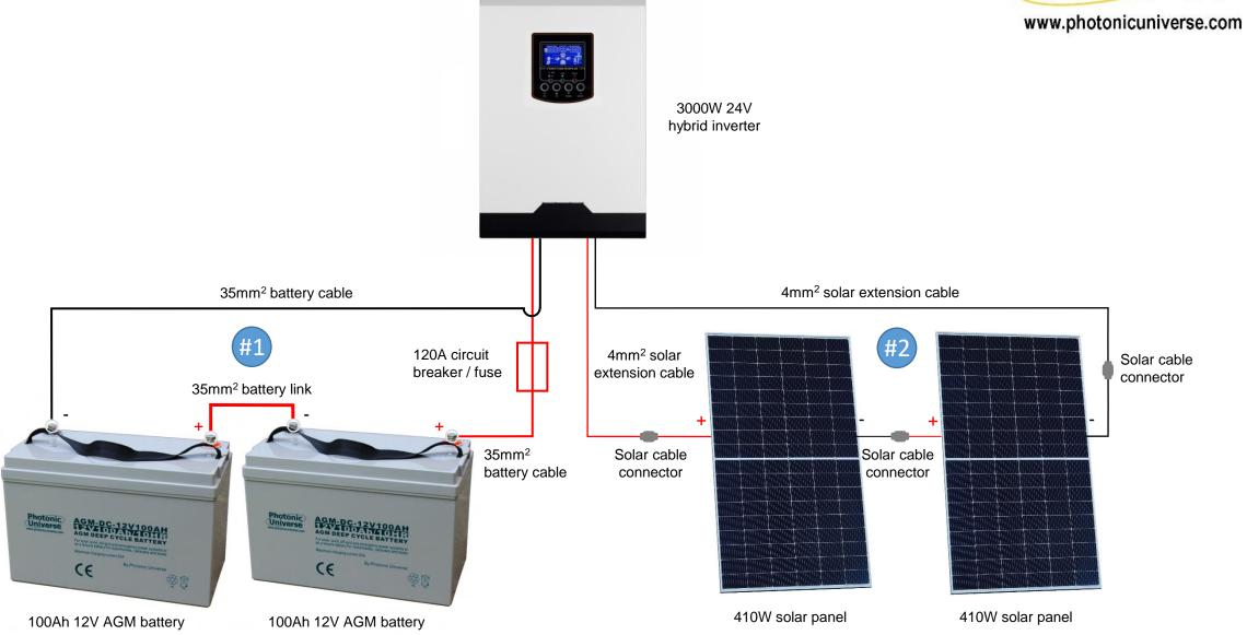
This wiring diagram is provided for general guidance only. For details on installation, wiring and mounting please refer to the user manuals and other technical documentation. Installation by an experienced and qualified person is required.
