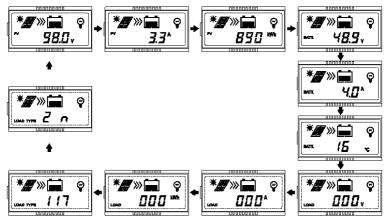
Note: When no operation, the display interface will be an automatic cycle except for the load time1 and load time 2 interface.
