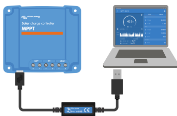
VictronConnect App connection via USB using a VE.Direct USB interface
