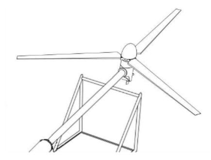
2. Fix the detachable part of the wind turbine connector to the top of tower by welding. Ensure that the centre line of the tower is parallel to the centre line of the casing when welding. Put the wind turbine head in the tower casing, and secure using the side screws.
